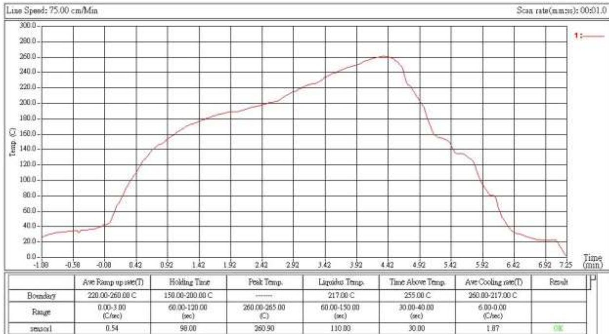
Figure 8.5 Solder Reflow Profile
