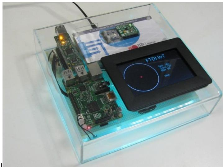
**Figure 1 FTDI IoT Demo Hardware**
